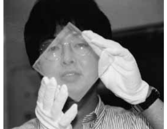
KEK physicist peers through a sample of aerogel, to be used for the Cherenkov counter in the Belle detector.
